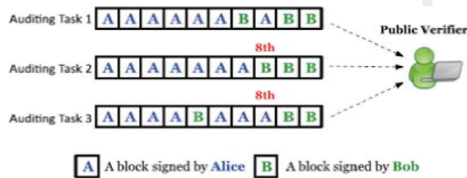
Fig. 1. Alice and Bob share a data file in the cloud, and a public verifier audits shared data integrity
