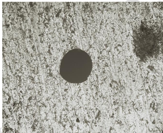
Fig. 9. SEM picture view of exit side of the machined hole (machining voltage of 18V, machining current of 3A, frequency of 120Hz, duty cycle of 40%).
