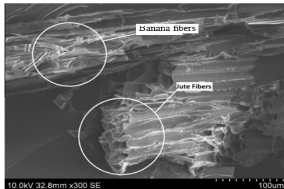
Fig. 14.SEM image of banana–jute–GFRP composite after tensile test
