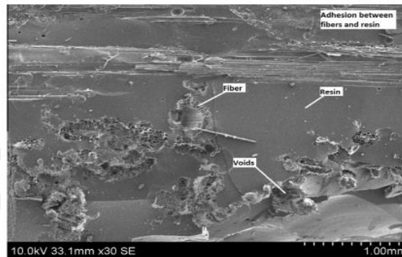
Fig. 13.SEM image of jute–GFRP composite after tensile test
