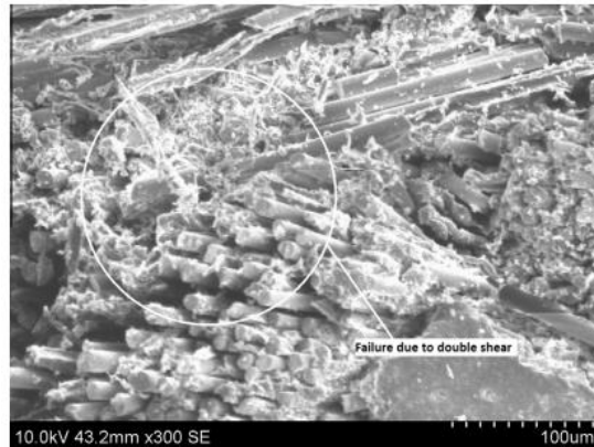
Fig. 15.SEM image of jute–GFRP composite after double shear test.
