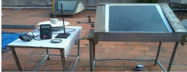
Fig 1. Pictorial view of the whole setup of cabinet solar still coupled with PCM
