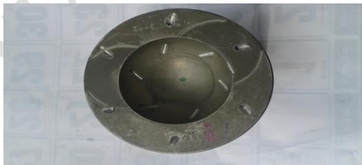
Fig. 1 Modified piston with 2.5 mm holes
