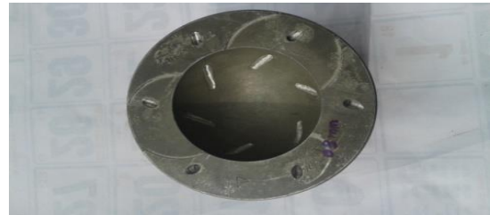
Fig. 2 Modified piston with 3 mm holes
