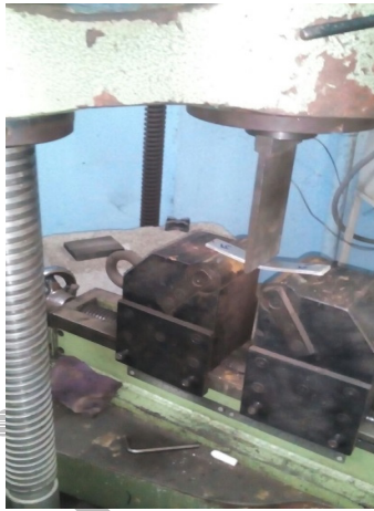
Figure 3. Machine used for Bending Test
