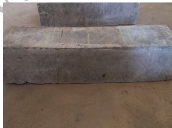
Figure 6 Ultimate load crack pattern
